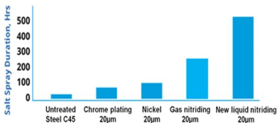
Corrosion resistance time measured according to ISO 9927 on a C45-type sample treated using various methods (exposure time before the first spots of red rust appear).
