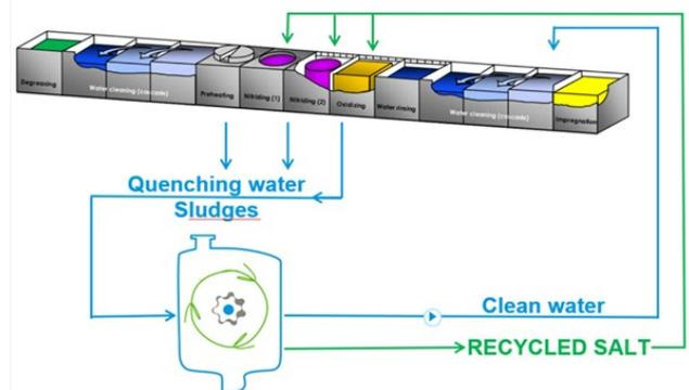
Reusing the salts obtained by recycling by-products on treatment lines results in the following:
