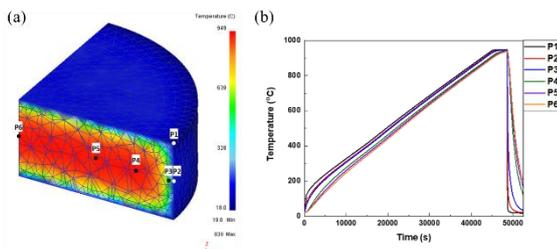
**Figure 2.** (a) Heat transfer analysis during solution treatment of the approximate size of an aero-engine disk of Ti64 and (b) P1~P6 point tracking during solution treatment.
