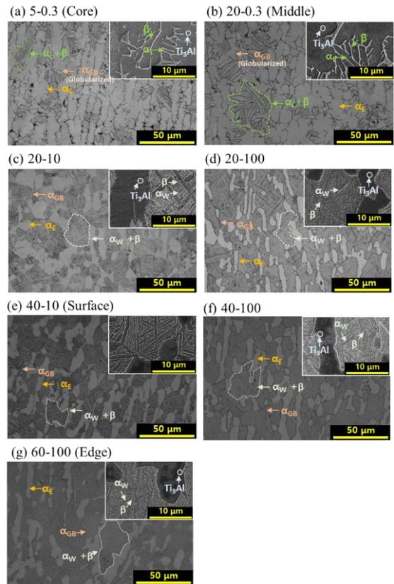
**Figure 3.** OM and SEM microstructures of STA heat treated samples with different solution treatment conditions of (a) 5-0.3, (b) 20-0.3, (c) 20-10, (d) 20-100, (e) 40-10, (f) 40-100, (g) 60-100.
